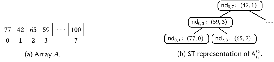
Fig. 5. ST representation with minima indexing. The entries A[4 : 6] are > 59 . The notation \text{nd}_{i,j} : (x, y) denotes \text{nd}_{i,j}.\text{min} = x , \text{nd}_{i,j}.\text{pos} = y .
